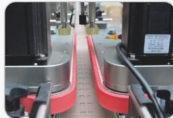
锁盖工位 Capping Station
