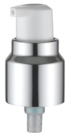
AGR 3010018(A/L) Specification: \varnothing 20/410 Discharge Rate: 0.20 \pm 0.03 \text{ ml/T}
