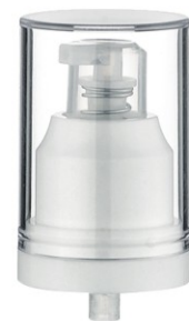
AGR 3010020(A/L) Specification: \varnothing 20/410 Discharge Rate: 0.20 \pm 0.03 \text{ ml/T}
