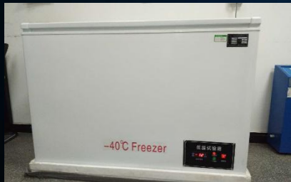
01 Low temperature tester
